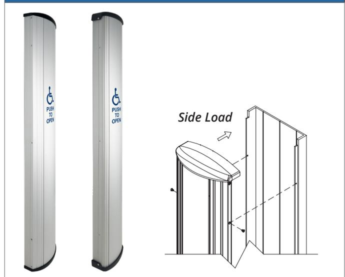
Camden **CM-84 & CM-85 Series** 'Side Load' Column™ push plate switches feature a two-piece construction with a surface-mount back box and are designed for use when an obstruction above the installed unit prevents the installation of a 'Top Load' model; where the Column™ switch is mounted to narrow curtain wall, or where the Column™ switch will span a lite of glass.
